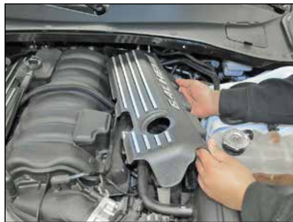
3. Lift up and remove the driver side ignition coil cover as shown.
