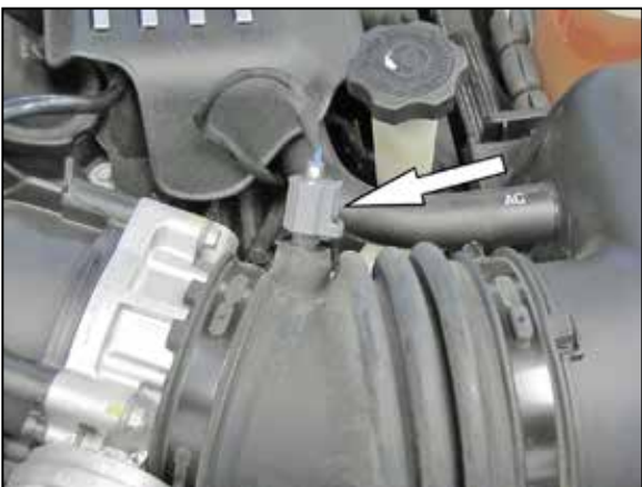
2. Disconnect the inlet air temperature air sensor electrical connection.
